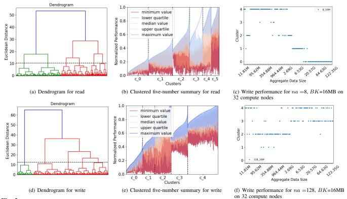
Fig. 2: Result Summary for the Statistical Benchmarking Method. In Figures 2(c) and 2(f), the x-axis is sorted based on the aggregate data size of an I/O pattern; the y-axis represents the cluster of a pattern.
