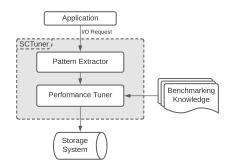
Fig. 1: Key components of SCTuner integrated into HPC I/O libraries
